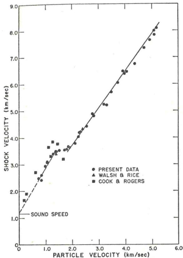
FIG. 6. Shock velocity-versus-particle velocity plot for carbon disulfide.
